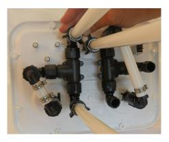
Connections shall be hand tight + ¼ turn. \*Do not over tighten as stress cracking may result.\*
