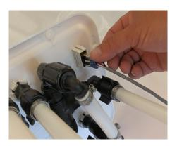
\*\*Make sure wiring connection is routed correctly for two switch operation.
