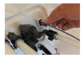
3. On back of switch, compress locking fingers on top. Push top side of switch through panel.
