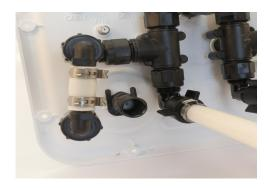
4. On back panel, insert thin flat head screwdriver under retainer clip securing **"WATER INLET."**
