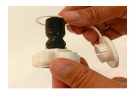
12. Dust cover should snap into front side of coupler without twisting dust cover strap.
