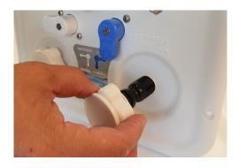
8. Remove and save dust cover on "WATER INLET." You will reuse it.
