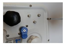
2. Disconnect power from back of pump switch.
