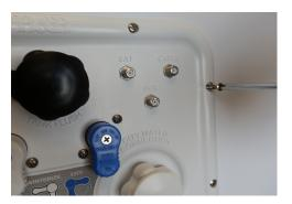
2. Remove coax line attached to connector you wish to replace.
