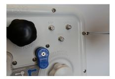
2. On back side of panel, unscrew plumbing line connected to diverter valve end labeled "TANK FILL."
