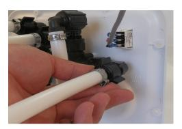
On back side of panel, unscrew plumbing line connected to diverter valve end labeled "TANK OUT."
