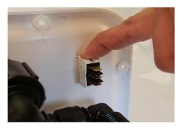
4. On back of switch, compress locking fingers on bottom. Push bottom side of switch through panel.
