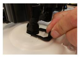
7. From front side of panel, pull **"WATER INLET"** out of panel.
