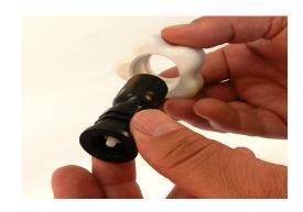
10. Insert new check valve into coupler.
