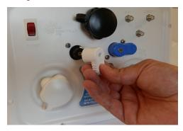
11a. Handle will turn clockwise to left facing position if installed correctly.
