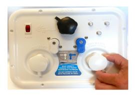
16. Screw plumbing line onto "WATER INLET." Hand-tighten + 1/4 turn.
