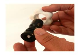
11. Assemble dust cover around check valve and back side of coupler.
