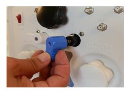
11a. Handle will turn counterclockwise to right facing position if installed correctly.
