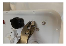
4. Wiggle connector back and forth while pulling to remove. Some unnecessary force may be required.
