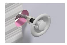
5. Position flange into cutout opening on sidewall & secure with (3) #8 self-tapping screws.
