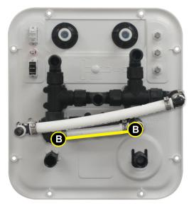
To connect fresh tank plumbing harness, screw swivel fittings onto diverter valves <sup>(3)</sup> (TANK FILL CITY & FROM TANK) as illustrated. This line will run directly to bottom of fresh water tank.
