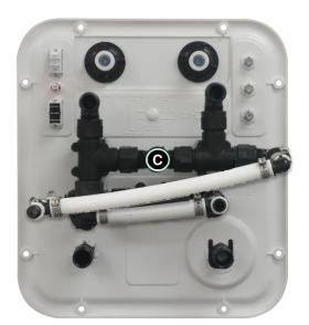
To connect plumbing line coming from pump, screw swivel fitting onto diverter valve **O** (PRESSURE FROM PUMP) as illustrated. This line will run directly to "OUT" side of water pump.
