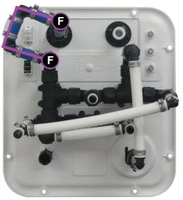
To connect the cold line plumbing harness, screw swivel fittings onto diverter valves (COLD, COLD LINE SUPPLY, & CITY TO FIXTURES) as illustrated. This line will connect to the cold water line feeding fixtures and water heater.
