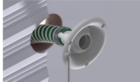
7. Position dish into cutout opening on sidewall & secure with (3) #8 self-tapping screws.
